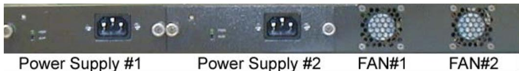
Figure 4. MX100-TG Gateway, Rear View
